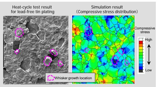
Hitachi, Ltd. and Renesas Electronics Corporation have codeveloped a simulation technology to simulate the whisker formation phenomenon, which may cause failures in electric and electronic devices. A whisker is the crystal-hillock extrusion occurring on lead-free tin plating.
